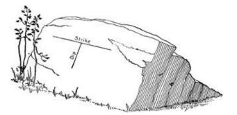
We first use the clinometer to find zero dip (this is the SAME as strike)! Keep moving across the rock face until the needle hangs at zero. We can then measure the dip angle (again using the clinometer) at right angles to the strike. The final measurement using the compass to find the direction in which the rock is dipping.
